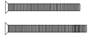
Flat Head Phillips Screw M5 x 55mm (2 1/8") L (3x) M5 x 65mm (2 1/2") L (3x)
